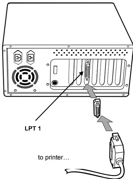
B. If computer is equipped with single parallel port then connect printer through hardware key using standard cable shipped with the printer.
