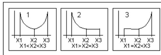
Simultaneously with peak border detection it is carried out baseline calculation that depends on parameter "Number of unresolved peaks" set by operator. This value must correspond to number of confident peaks merged into group (see 4.12).
