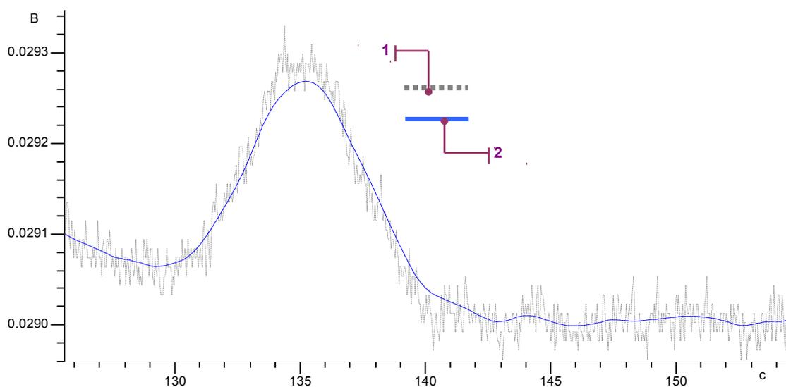
The spikes removal is the sort of data smoothing. This data processing element removes only high-frequency signal splashes caused by power supply instability, flame - ionization detectors flame instability etc. When the peak width is significantly greater than high-frequency spike width, the peak area and hight wont be affected. Spikes removal may be used to simplify tuning of the peak-detection algorithm and increase the quality of signal integration.
