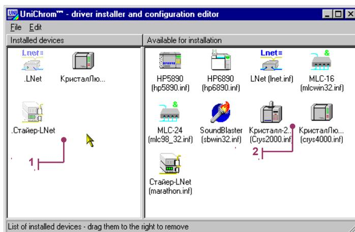
The working field of this program consists of two parts. In the left part it is placed icons of already installed devices. In the right part is presented icons of devices which are available for installation. Device is installed and ready to work when all drivers for that device are installed and configuration is written to System Registry.
