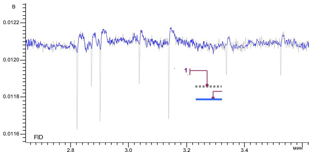
Into UniChrom are incorporated five standard smoothing methods (linear over 3 or 5 nodes, 3-rd order polynomial smoothing over 5, 9 and 11 nodes), spline interpolation, one proprietary algorithm, two spike removal algorithms and also other special algorithms. All the mentioned data processing methods can be applied either to the whole signal as to the fragment of signal (between markers).
