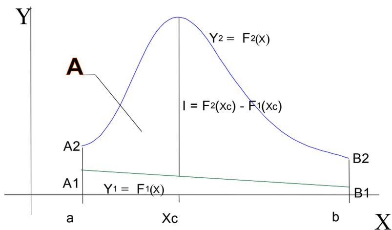
When calculated peak area is less than limit set by "minimal area" or determined peak intensity less than "Noise level" both set by operator, then this peak is excluded. So varying of parameters "Area limit" and "Noise level" operator can affect on peak detection sensitivity.
