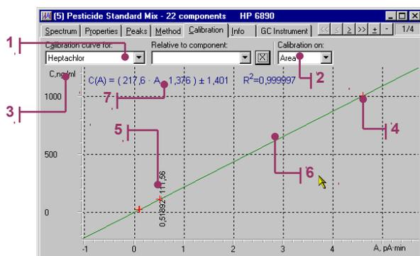
For using external standard calculation method it is a need to build the calibration sequence, which states the relation between height and area (detector response) to substance concentration. The calibration procedure is taken automatically when operator marks components of standard mixture as "external standard".
