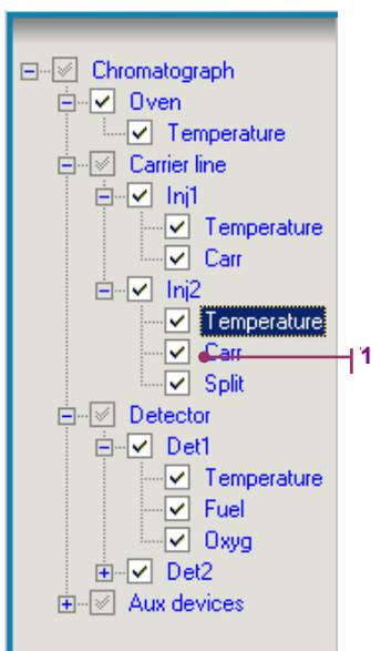
In most cases the quantity of software regulators is much greater than number of physical regulators installed in the instrument. When the program connects to the working instrument, the non-existent regulators would be hidden. Show or hide the software regulator is possible at any moment with single click in shown at 2.5.1.1 area of regulators panel. Being shown the regulators are displaying the actual values and allow the alteration of the values.
