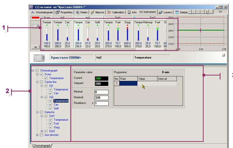
The panel of control zones displays in compact form the actual state of all temperature and gas control zones simultaneously. The panel allows with the single click move from one regulator settings to another's.
