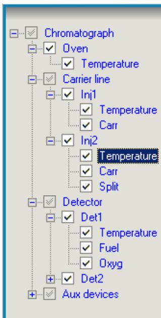
There are instruments with auxiliary (non standard) heating zones and flow control zones. For supporting such instruments in UniChrom added three auxiliary zones, each one with one thermal and one gas regulator.
