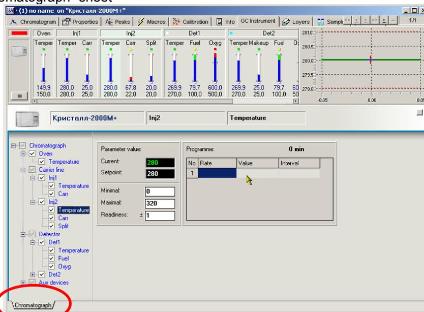
At the page Chromatograph always shown the ACTUAL instrument state. I.e. information about instrument state periodically read from the instrument and displayed in all the panels. Any alteration of the instrument settings at this page are immediately going to chromatograph.
