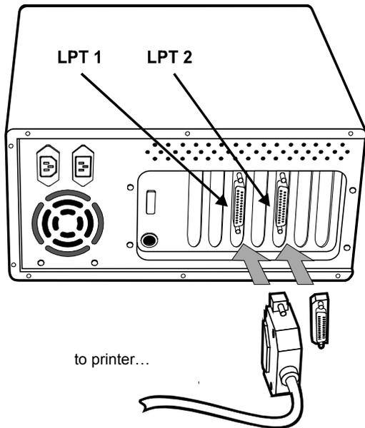
A. Connect electronic security key of UniChrom system to the spare printer port of computer – parallel port IEEE-1284 standard with connector of type B (D25). Connect the printer to second spare parallel port according to printer manual.
