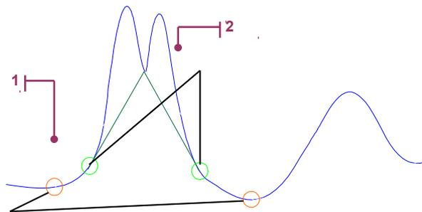
Used in UniChrom peak detection algorithm is a standard peak detection method (see. McCloskey D.H., Hawkes S.J., "J. Chromatogr. Sci.", 13, 1, 1975), adopted for processing of signals with high noise level. Processed real chromatogram fragments from different GC devices (see 4.12).
