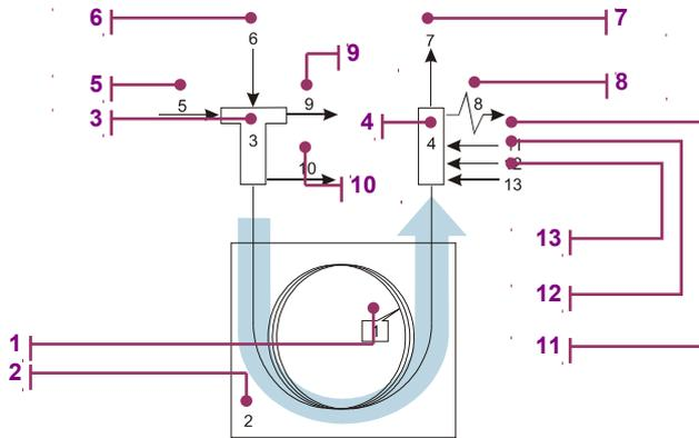
Now there are five regulators: split flow, septum (rubber plumb) purge flow, detector makeup gas, hydrogen flow and air flow. The first and second flows are logically bound with inlet, the rest flow regulators bound to detector zone.
